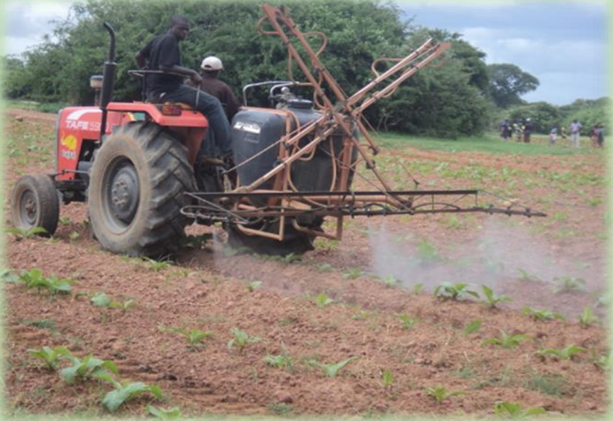
Photo 12. Spraying Tobacco Pesticides in Tobacco Field with Tractor Mounted Sprayer Boom
